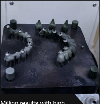
Milling results with high surface quality
